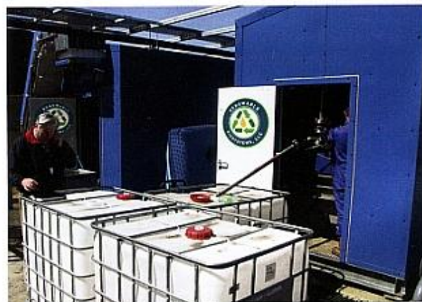
Oil totes are filled and sent to their destination, such as a nearby biodiesel plant for further cleaning and processing into fuel.
