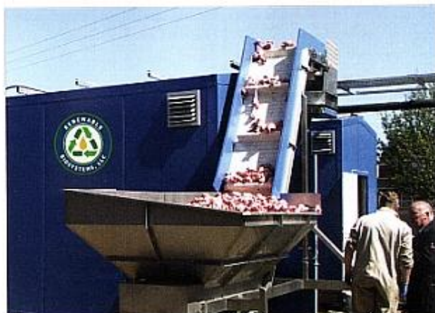
Renewable BioSystems' oil extraction machines, which employ particle-size reduction, heat and centrifugation, are sized to process between 3 and 15 tons per hour.
