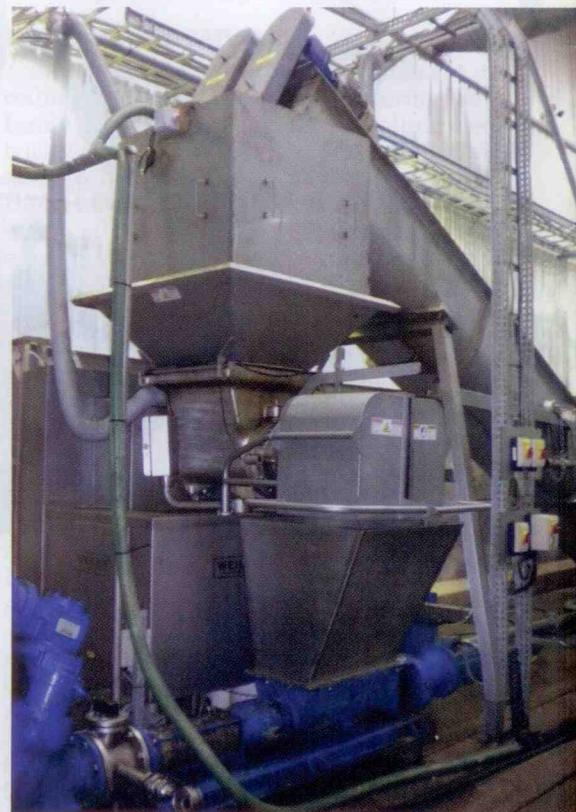
Organic wastes are fed into the extraction system's macerator (above), which forms a slurry. A centrifuge separates the slurry into oil, wastewater and solids (right).
