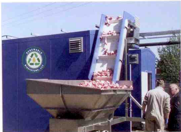
Renewable BioSystems’ oil extraction machines, which employ particle-size reduction, heat and centrifugation, are sized to process between 3 and 15 tons per hour.
